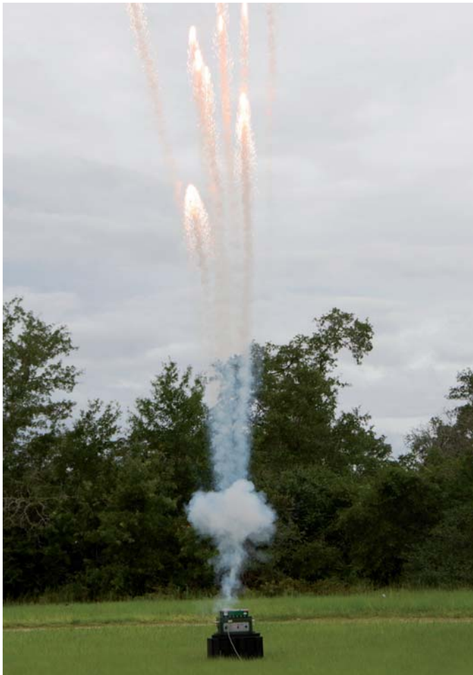
White Star, Target Hit Cartridge (M35) simulates the effect of a steel on steel hit or a large calibre munitions explosion.
