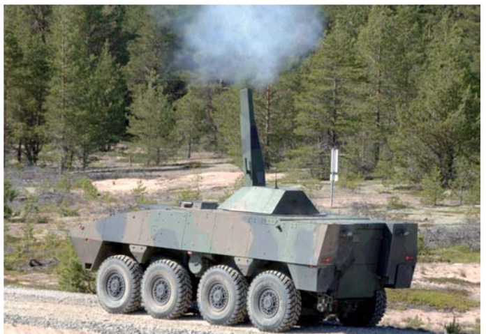
Patria's NEMO firing Mearc 120mm mortar ammunition.
