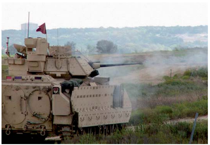
Bushmaster cannon firing 25mm ammunition.
